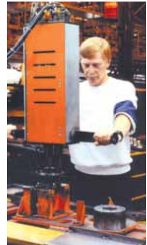
Repair bay operator is using a two spindle fixtured tool to fasten components of a wheel hub assembly.
