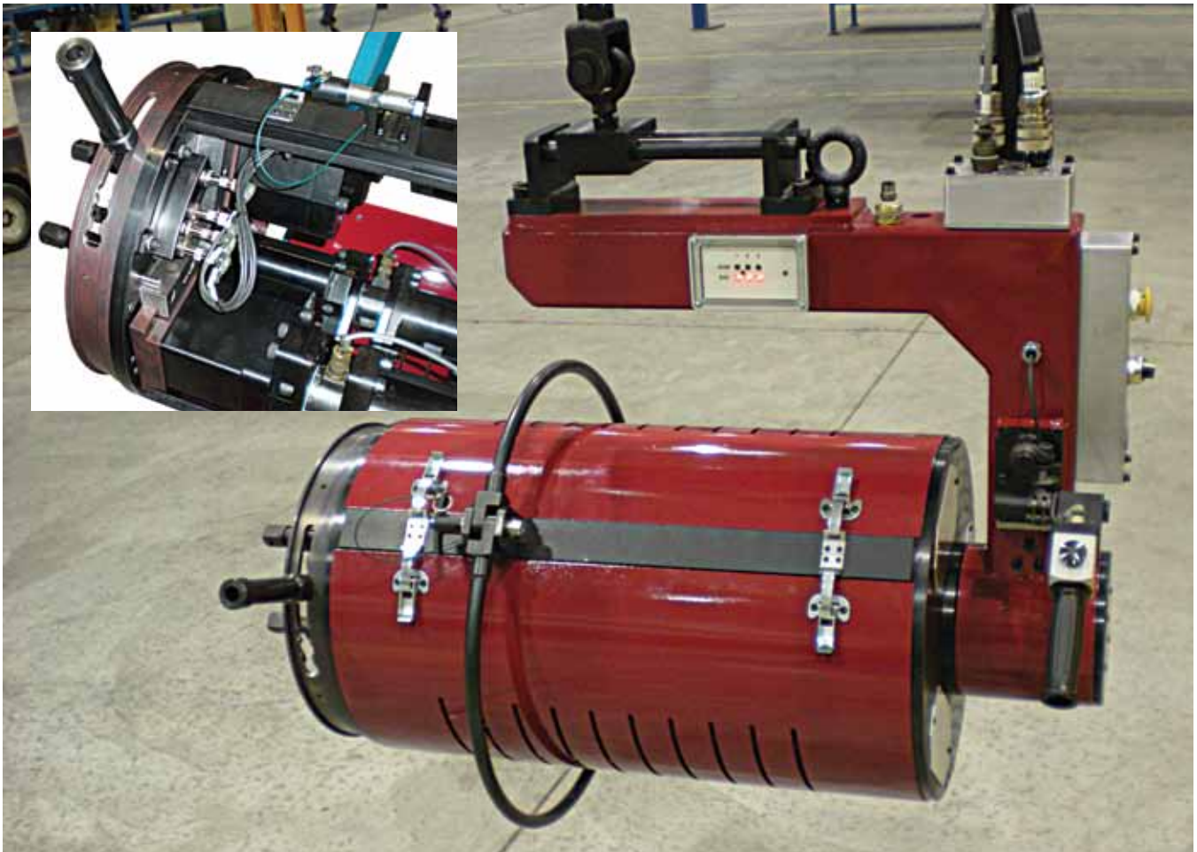
The above manually operated railroad wheel bearing multiple has the capability to tighten three (3) fasteners equally spaced on various centers between 3.50" to 5.85" diameters up to 600 NM torque.
