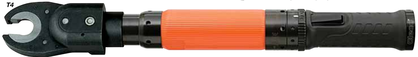
The 48ET tube nut wrench alternates the direction of rotation each time the lever is actuated. When rotating in reverse, the socket will stop at the open position.
